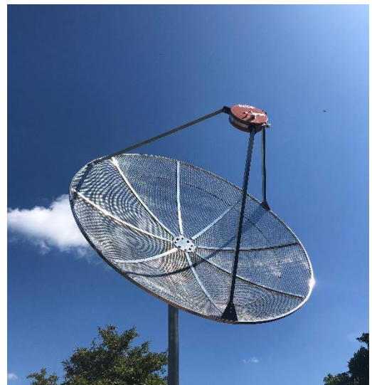
1M2 RF HAMDESIGN DISH & Dual Band Es-Hail 2 Dish feed
