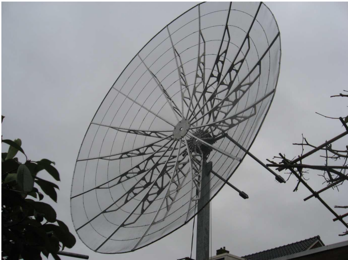
Picture 4.5 Meter Mesh Dish (6mm Mesh, max 6GHz)
