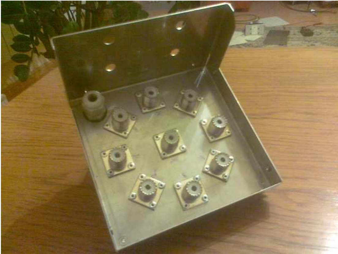
Photo 2. Antenna Relay PANT-8 NEW ver.11/2012 view from the sockets UC-1 side
